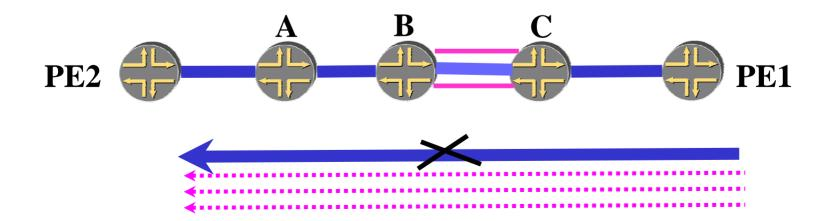
Make-before-break – set up a new path before tearing down the old path
